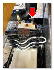
Use a gauge to make sure the hydraulic pressure is set at 2500 psi for trailer units or 3000 psi for PTO units.
