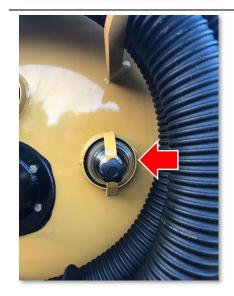
Remove the sight glass located on the right side of the debris tank door.
