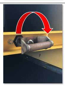
Turn the lock bar handle ½ turn clockwise at a time until the lock pin is in the center of the bracket hole.
