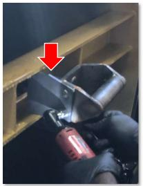
If the pin is not centered, open the door and remove the lock plate from the lock bar.
