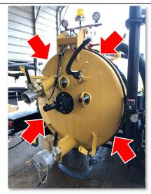
Feel all around the door seal to make sure all leaks have been stopped.
