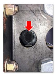
Look through the sight glass opening to ensure the lock pin is in the center of the bracket hole.
