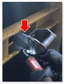
Replace the lock plate, close the side door, and replace the sight glass.
