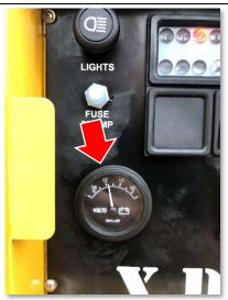
Check that the battery is supplying between 12-14 volts.
