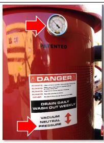
Turn on the reverse pressure with the door locked. The pressure should read between 3-5 psi.
